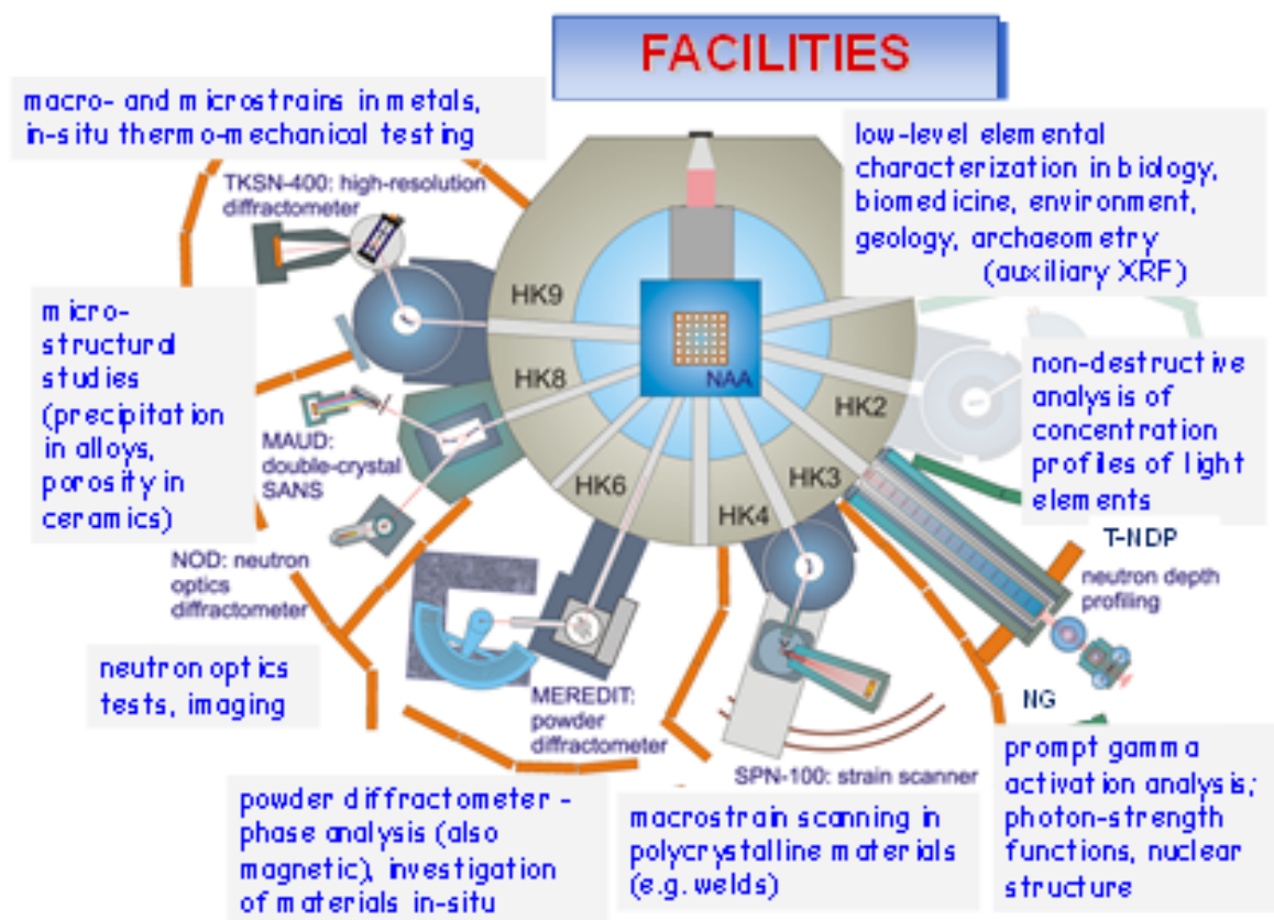
Fig. 1 Schematic picture of the experimental facilities of NPL at the reactor LVR-15
