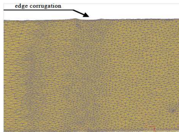
Fig. 13 The defect of round hole type (No. 05) located sideways, after rolling at deformation temperature of 1200°C and 50% deformation
