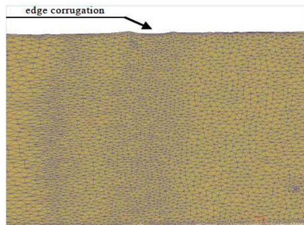
Fig. 14 The defect of round hole type (No. 06) placed sideways, after rolling at deformation temperature of 1200°C and 50% deformation
