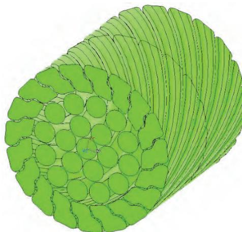
Fig. 2 Z-geometry of steel rope
