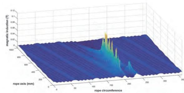
Fig. 10 Magnetic field distribution around steel rope with multiple wire cracks according to Fig. 9
