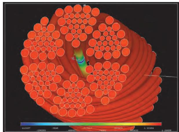
Fig. 7 The geometry of inner wire crack (1 mm gap)
