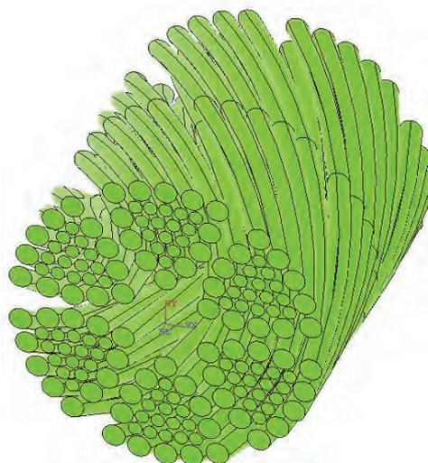
Fig. 1 Cross-section of six strands rope combining thick and thin wires
