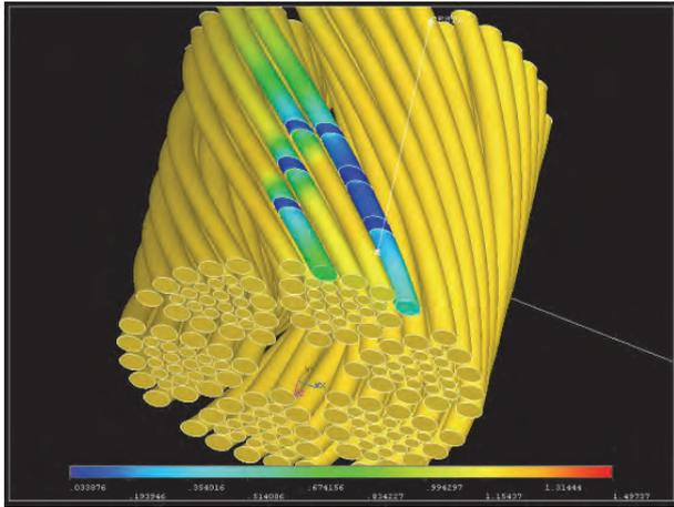
Fig. 9 Steel rope with multiple wire cracks
