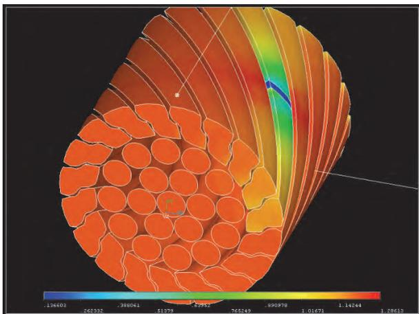
Fig. 11 Z-geometry rope with surface breakage
