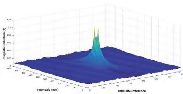
Fig. 4 3D distribution of secondary magnetic field for wire crack (1 mm) on the rope periphery (six strands rope) according to Fig. 3
