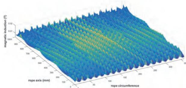
Fig. 14 Modulation of the magnetic field around Z-shape rope by internal crack according to Fig. 13
