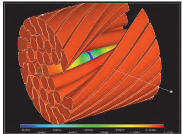
Fig. 13 Steel ropes with a Z-geometry with internal crack
