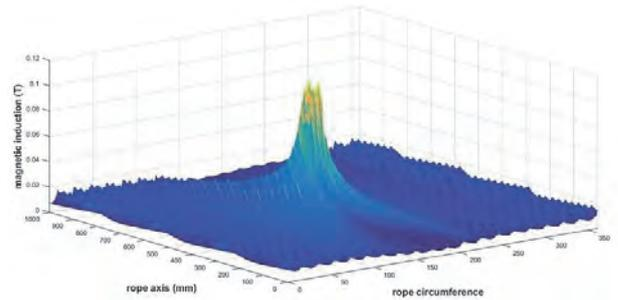
Fig. 12 Magnetic field modulation for Z-geometry rope with surface breakage according to Fig. 11
