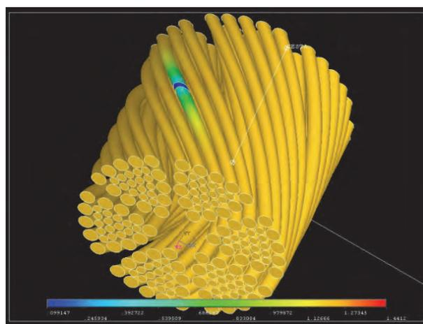
Fig. 3 The rope with a surface defect; the positions of the defect is specified by colored fronts of wire
