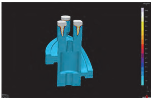
Obr. 3 Porozita odlitku Fig. 3 Porosity of casting
