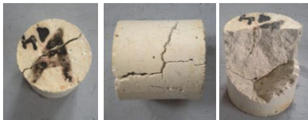
Fig. 7 Reference sample "A" burned at 1400 °C at disintegration after 16 cycles
