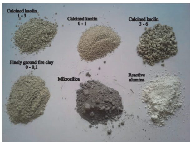
Fig. 2 Fillers of the mixture – three fractions of calcined kaolin, finely ground fire clay, micro-silica and reactive alumina
