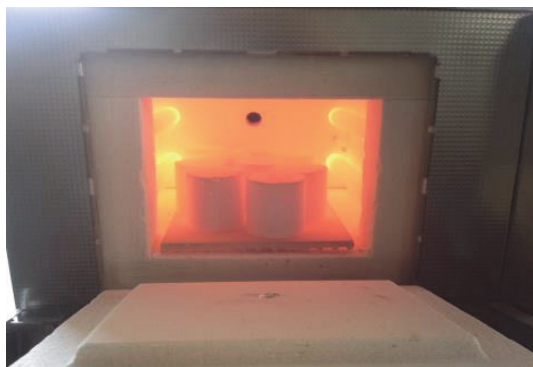
Fig. 6 Test samples in the furnace during the experiment on resistance to sudden temperature changes
