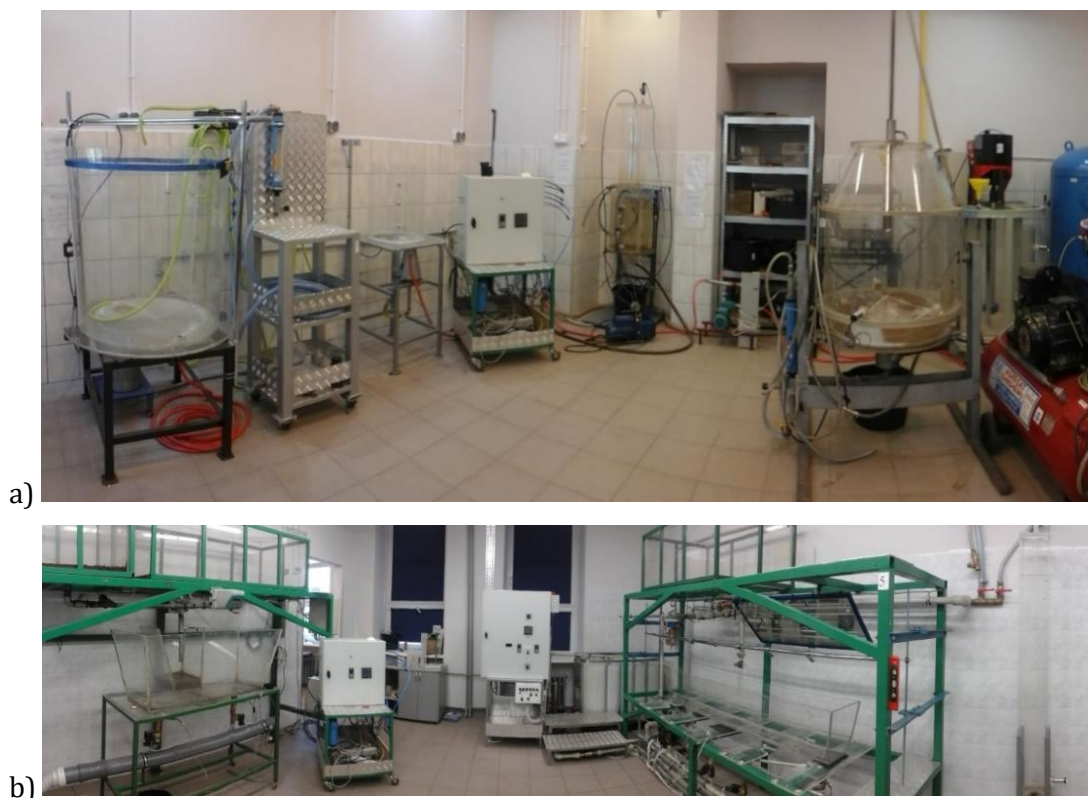
Fig. 2 View of the Metallurgical Process Modelling Laboratory: a) models of the oxygen converter, ladle furnace and RH device, b) models of the CSC and crystallizers
