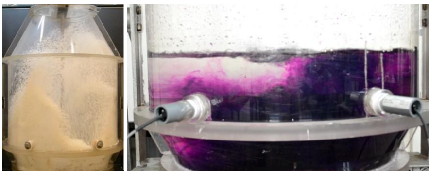
Fig. 3 Visualization of the flow of the model liquid in the oxygen converter
