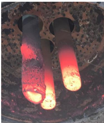
Obr. 3 Pohled na trysku ve víku LF Fig. 3 View of the lance in the LF cover
