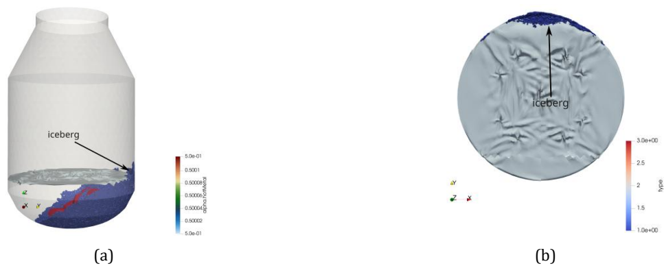
Fig. 4 Iceberg formation near the furnace wall as a result of simple rocking furnace leading to uneven distribution of scrap (colored by type Red for heavy, gray for medium and blue for light) at the end of the furnace rotation and prior to the blowing stage. (a) the side view of the furnace, (b) the top of the scrap hot metal interface (colored by volume fraction)
