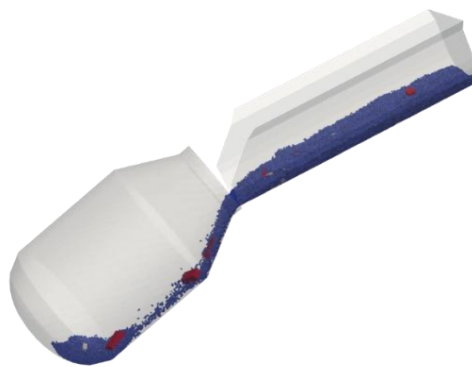
Fig. 1 Horizontally packed scrap of three types namely heavy, medium, and light (colored red, gray, and blue, respectively) being discharged from the scrap box into the converter
