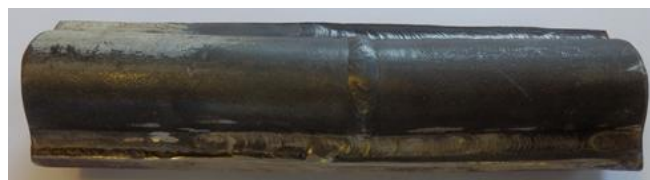
Fig. 7 Photo of the welded on the T24 \alpha -Fe pipe
