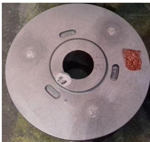
Fig. 1 Type of casting used to assess the occurrence of shrinkage
