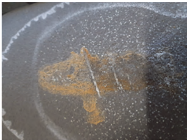
Obr. 3 Vady povrchu elektrody 5A Fig. 3 Electrode 5A surface defects
