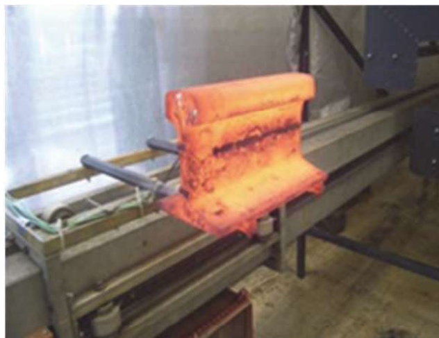
Fig. 6 Diagram of the laboratory test rig for designing and optimization of cooling sections for rolled products
