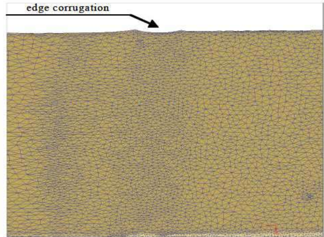
Fig.10 The defect of U-shaped notch type (No.02) oriented transversely, after hot rolling at deformation temperature of 1200°C and 50% deformation
