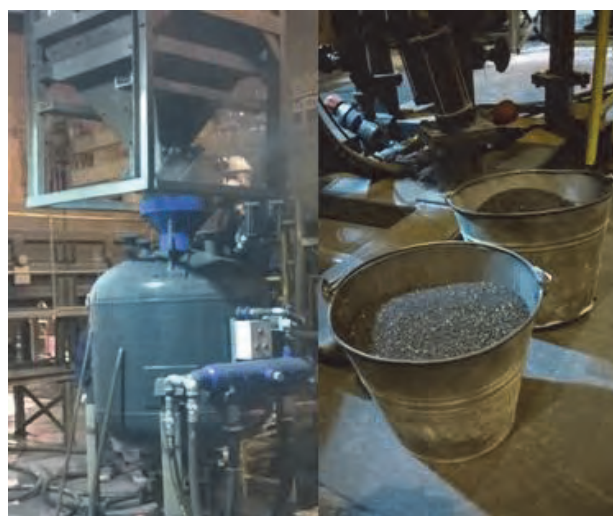
Fig. 6 Filling up the pressure vessel with reduction agents
