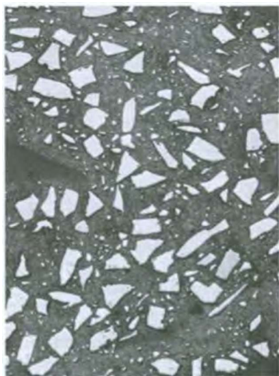
Obr. 3 Mikrostruktura kompozitu \text{SiC} v \text{Al} matici Fig. 3 Micro-structure of \text{SiC} composite in \text{Al} matrix
