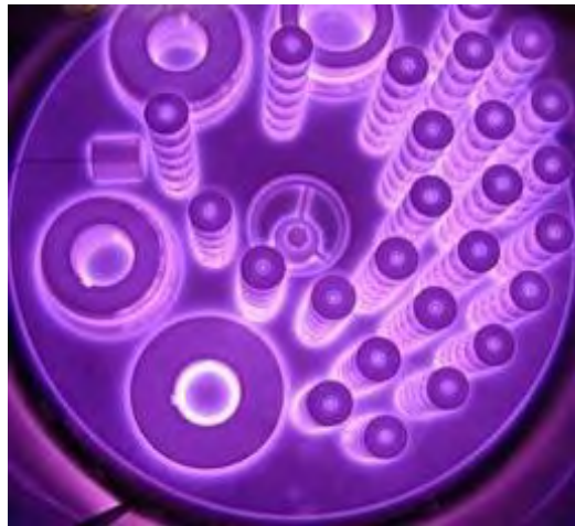
Obr. 2 Výboj během nitridace, tzv. Eliášovo světlo [5] Fig. 2 Discharge during nitriding (so called Elijah's light)
