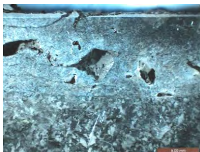
Obr. 10 Detail studených spojov a defektov v povrchovej kôre na širokej stene, vzorka 1B1 Fig. 10 Detail of cold joint and defects at shell surface on wide face, sample 1B1
