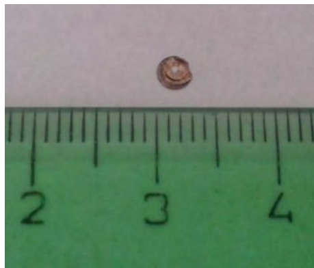
Obr. 6 Tenká kovová fólie vzorku AII Fig. 6 Sample AII for TEM analysis
