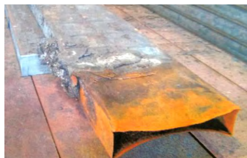
Obr. 1 Prievalová brama Fig. 1 Breakout slab
