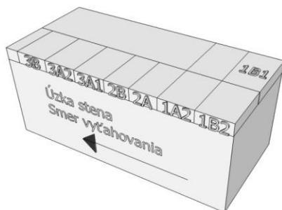
Obr. 3 Schéma odberu vzoriek z mikroprievalu Fig. 3 Cut-outs from the bleeder sample
