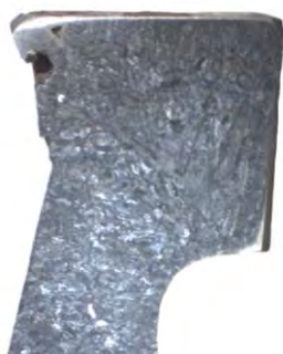
Obr. 29 Priečný rez rohu zliatku, vzorka LS 3 Fig. 29 Cross-section of the corner from the breakout shell, sample LS 3
