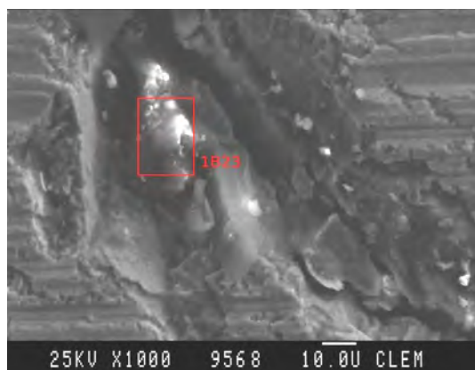
Obr. 18 REM z oblasti trhliny, vzorka 1B1 Fig. 18 SEM of the crack area, sample 1B1
