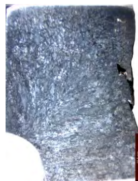
Obr. 30 Priečný rez rohu zliatku, vzorka LS 6 Fig. 30 Cross-section of the corner from the breakout shell, sample LS 6
