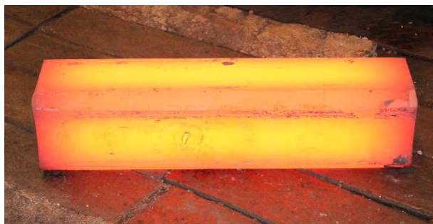
Fig. 7 \square 205\text{mm R40} billet edge after calibration
