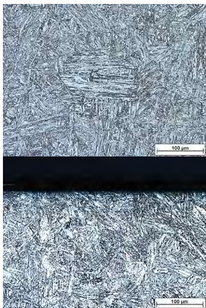
Fig. 1 Microstructure and character of corrosion attack for steel COR 13-4
