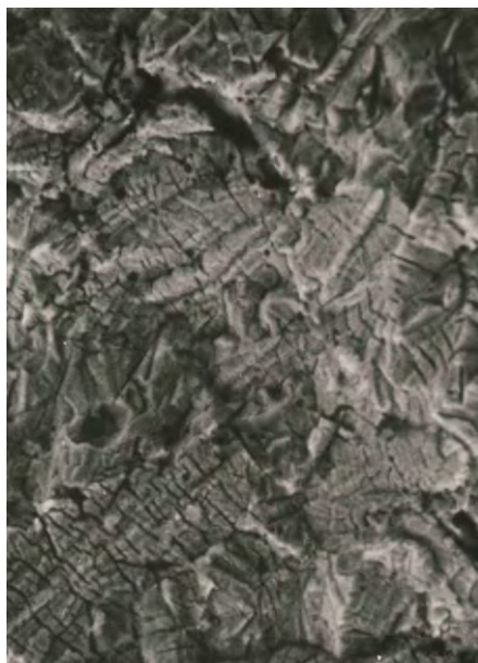
Fig. 9 Micromorphology of bolt fracture surface, REM, zoomed 1000x
