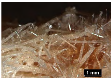
Fig. 4 LOM image of the needle-like single crystal of ZnO (sample No. 4)
