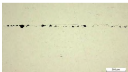
Fig. 6 Macroinclusions – basic material of the damaged shaft – cut in the longitudinal direction; zoomed 100x
