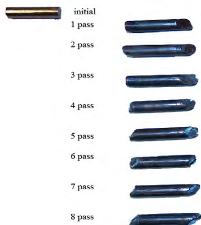
Fig. 4 Copper samples after individual passes with use of the ECAP technology
